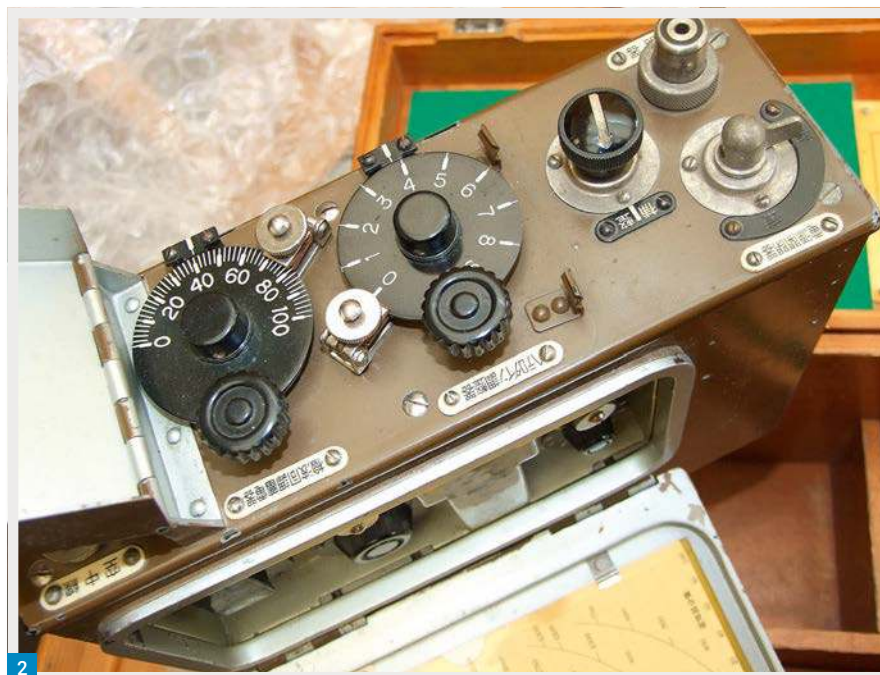
Fig. 1: The Japanese 53C receiver. Fig. 2: The two tuning controls. Fig. 3: The circuit diagram.
