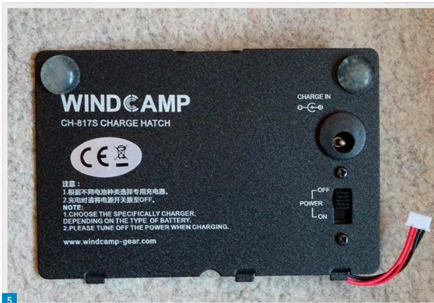
Fig. 5: The alternative Windcamp battery cover required when using a Windcamp WLB-817S battery. Fig. 6: The small JST connector used to connect the battery on a Yaesu FT-817.
