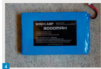
Fig. 1: A 'genuine' Yaesu FNB-85 NiMH battery rated at 1400mAh. Fig. 2: An 'equivalent' to the Yaesu FNB-85 NiMH battery advertised on Amazon. Fig. 3: The Yaesu battery box with eight AA 2000mAh NiMH cells from Amazon. Fig. 4: The Windcamp WLB-817S is a 3000mAh LiPo battery.
